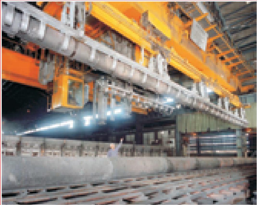
Graphite electrodes being loaded in a LWG furnace.
